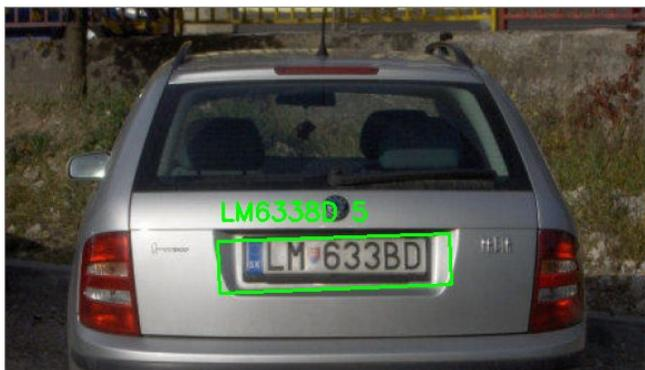
Figura 3. Prueba con OpenCV OCR and text recognition with Tesseract.
