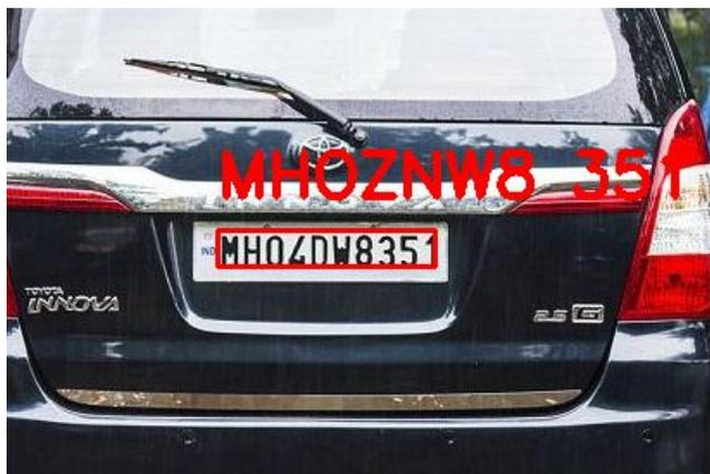
Figura 5. Prueba con OpenCV: Automatic License/Number Plate Recognition (ANPR) with Python.
